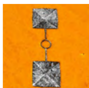
MFM mode, Soft magnetic nanostructures, 25µm scan
